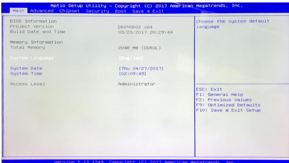
3 of 8. The rest of the steps will use the keyboard only. Please use the navigational keys (←,↑,↓ and →) to move around and the “ENTER” key to make a selection. Navigate to and select the “Advanced” tab then go to and select “System Component”:
