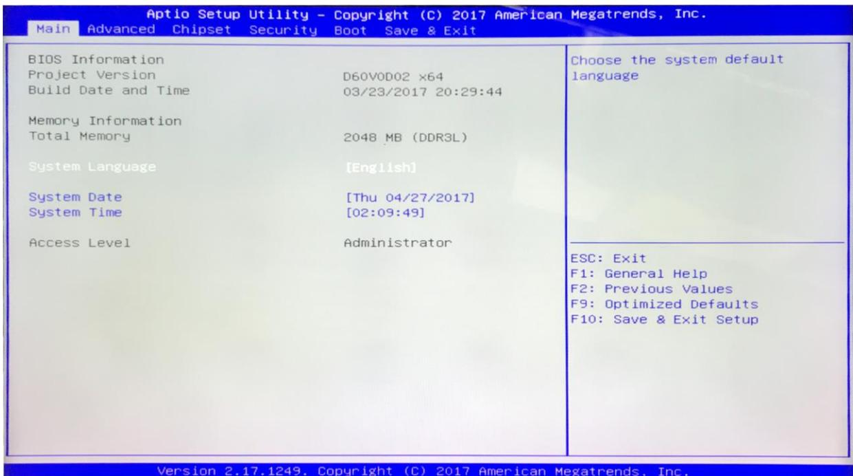
3 of 8. The rest of the steps will use the keyboard only. Please use the navigational keys (←,↑,↓ and →) to move around and the “ENTER” key to make a selection. Navigate to and select the “Advanced” tab then go to and select “System Component”:
