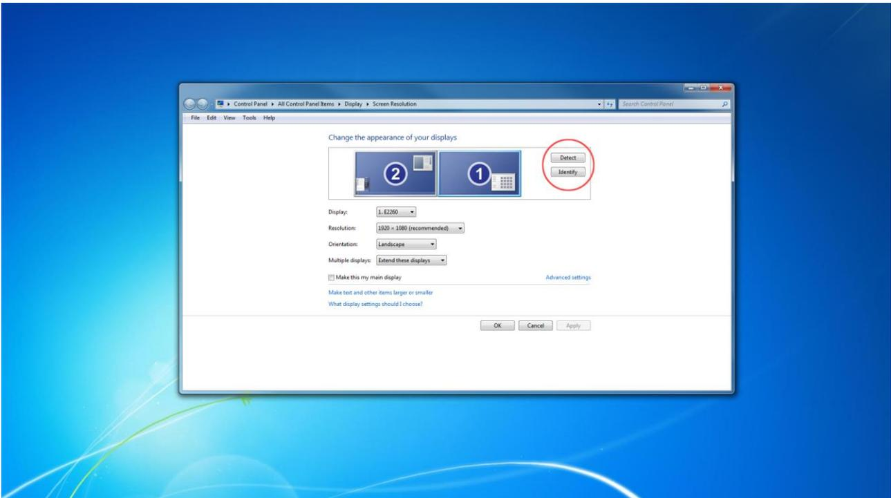
Select the display that corresponds with the Video Monitor display then check the box “Make this my main display” or “Use this device as the primary monitor”. This will make the Video Monitor display your main monitor.
