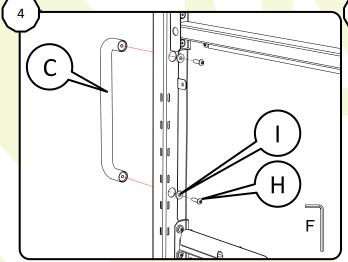
Assemble the handle to the frame (● 5 mm)
