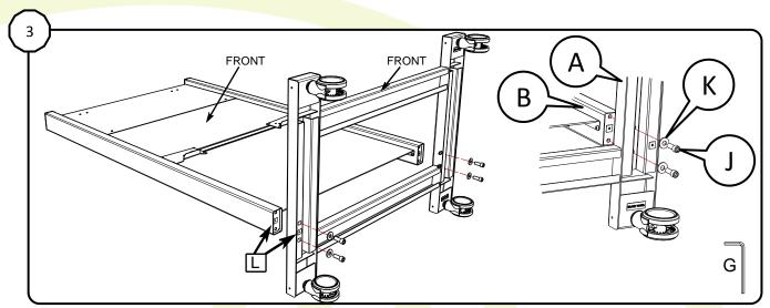
Assemble wheelframe (A) and top frame (B) from the bottom. Match the left (L) and right (R) labels on wheelframe and topframe, tighten well (● 10 mm)
