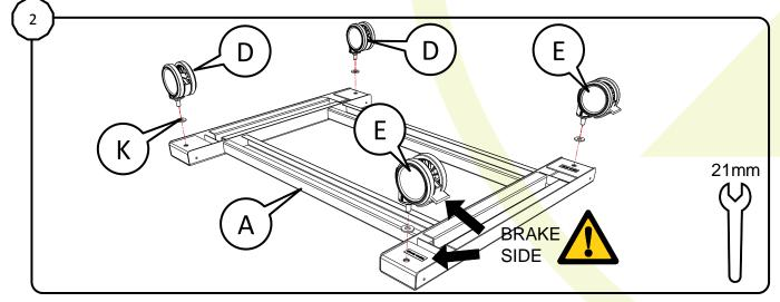
Assemble the wheels on the wheel frame (21 mm wrench), note wheel E with brake goes on the side with the sticker.
