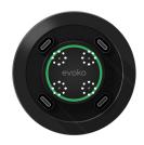
Press and hold any of the touch buttons for 5 second until a white light appears at port 4.
