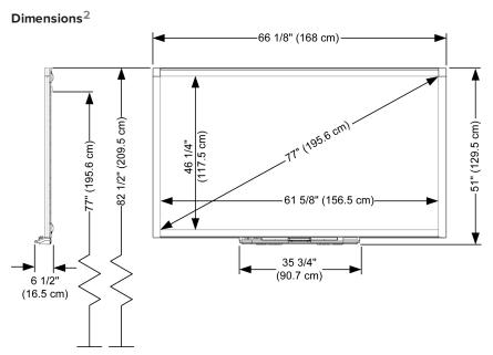
Leave at least 5/8" (1.6 cm) headroom to wall mount the SB880. The distance from the bottom of the wall mount bracket to the top of an installed interactive whiteboard is 6 1/8" (15.6 cm).
